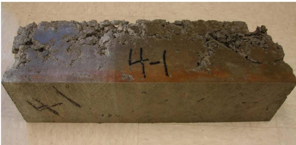
FIGURE 10. LAB 4 BEAM 1 VOIDS AND POOR CONSOLIDATION
