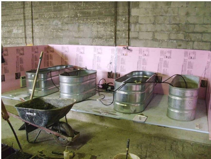
FIGURE 3. CURING TANKS SHOWN WITH SINGLE PUMP RECIRCULATION SYSTEM INSTALLED
