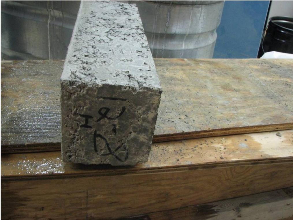
FIGURE 9. LAB 12 BEAM WITH KNOWN VOIDS AND POOR CONSOLIDATION
